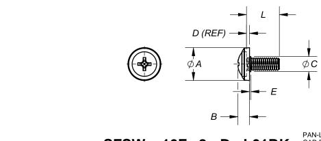
PAN-L-SCREW, .190-32 UNJF-3A x 1/2" LG, L01BK = PART NO. EXAMPLE: SFSW CAD PLT, PHILLIPS DRIVE, LUSTERLESS BLACK PER FED-STD-595, COLOR #37038 - COLOR - SEE STOCK COLOR LIST DWG. NO. SCL870115
