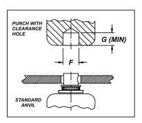
Table 1 below for recommended punch clearance hole size. Due to the wide variety of press equipment available and the simplicity of the punch and anvil required, it is intended that customers fabricate their own
