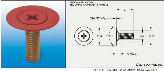
PART NO. EXAMPLE: FCM 10F 10 S03RD .190-32 X 5/8" LG, STEEL, PHILLIPS DRIVE, SEMI-GLOSS RED PER FED-STD-595 NO. 21105 +.00 DIM DATA **LENGTH THREAD** TOLERANCE ±.02 **HEAD COLOR** MATERIAL **TYPE** CODE 5  $\frac{1}{4}$  $\frac{3}{8}$ <u>5</u> 8 A В D CODE 1 C SIZE 16 16  $\frac{1}{2}$ 8 .138-32 6C 7 4 5 6 8 10 12 14 16 .50 .18 .30 .13 UNC-3A SEE D STOCK .164-32 COLOR **FCM** 8C 4 5 6 7 8 10 12 14 16 STEEL 56 21 36 14 UNC-3A LIST **PHILLIPS** Doc No. DRIVE SCL870115
