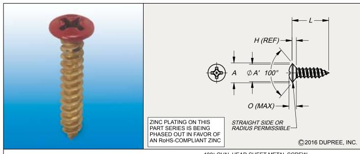
PART NO. EXAMPLE: OH 6SM 12 D G03RD = 100° OVAL HEAD SHEET METAL SCREW, 6-20 X 3/4" LG, STEEL, PHILLIPS DRIVE, GLOSS RED PER FED-STD-595 NO. 11105
