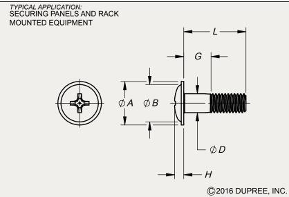
PART NO. EXAMPLE: WH 10 R10 D S15BG = WASHER HEAD SCREW, .190-32 UNF-3A X 5/8" LG, 7/32" GRIP, ALLOY STEEL, CRUCIFORM RECESS, SEMI-GLOSS BEIGE PER FED-STD-595 NO. 27722
